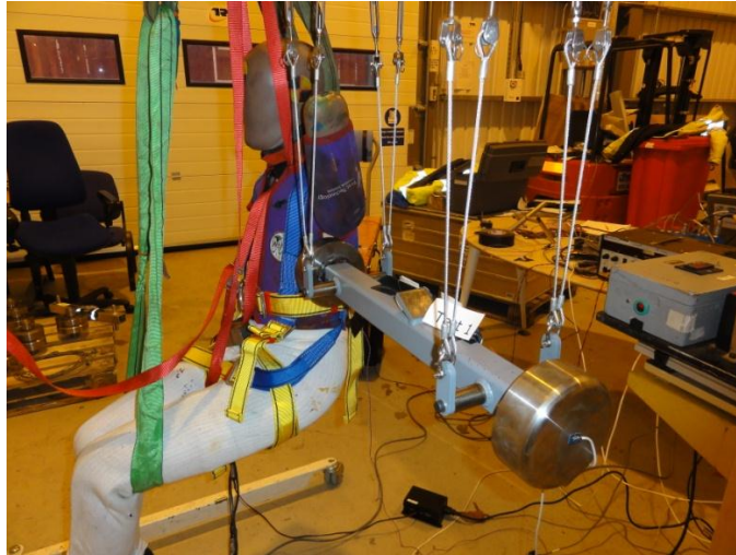
Figure 3-6: Impactor test configuration from the lateral thorax impacts as conducted by UMTRI
