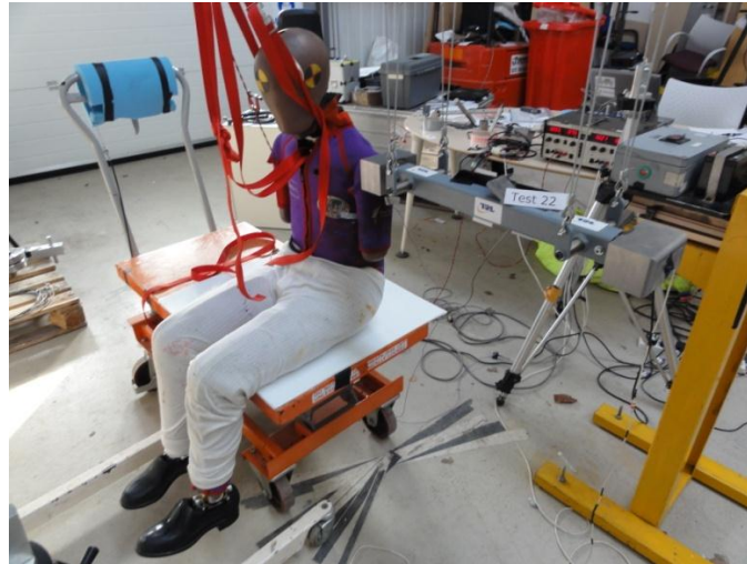
Figure 3-1: Impactor test configuration from the lateral and oblique-lateral shoulder impacts conducted by INRETS
