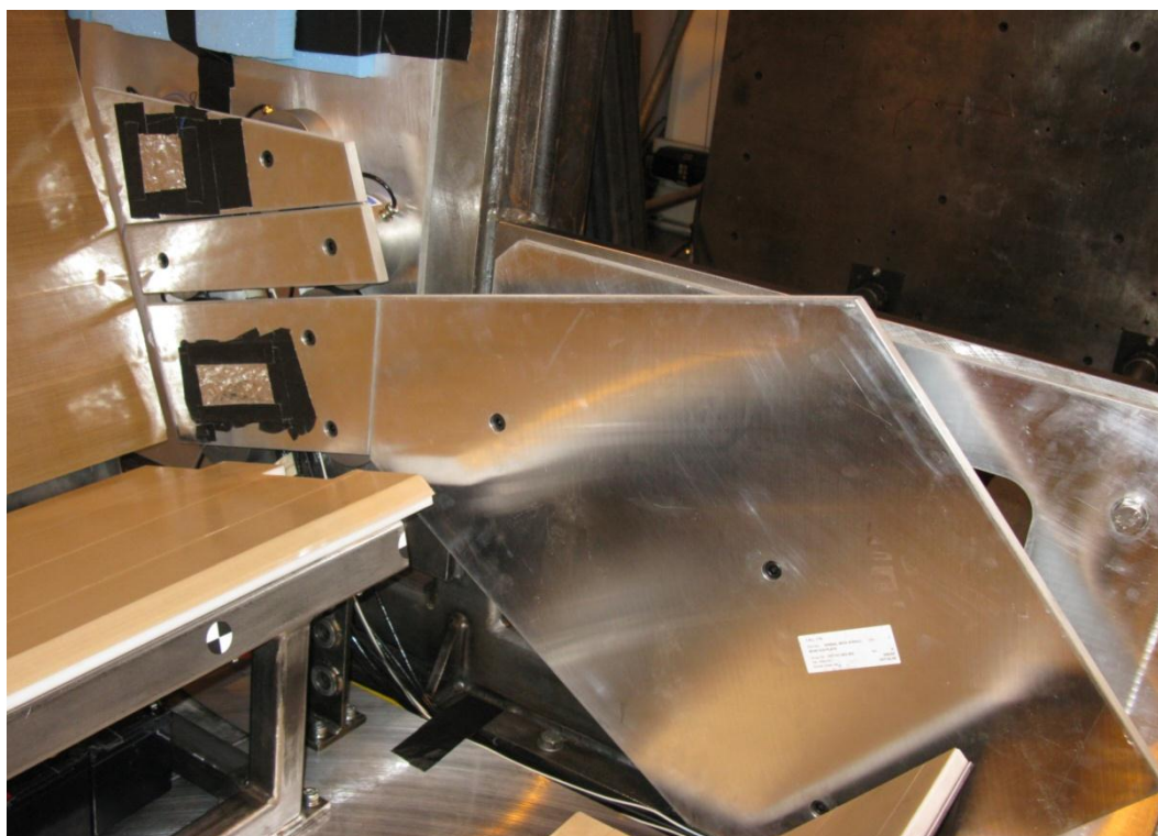
Figure 3-13: MCW/VRTC side impact buck showing load plates for the thorax, abdomen, pelvis and leg
