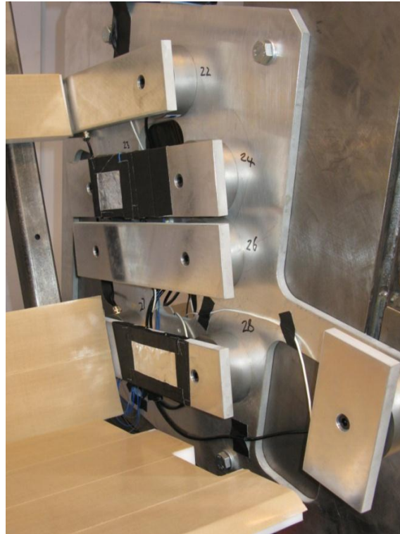
Figure 3-12: WSU side impact sidewall showing beams at four levels plus knee load plate
