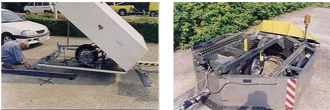
Figure 4.3: Examples of CPX noise measurement vehicles from Austria (left) and Germany (right)
