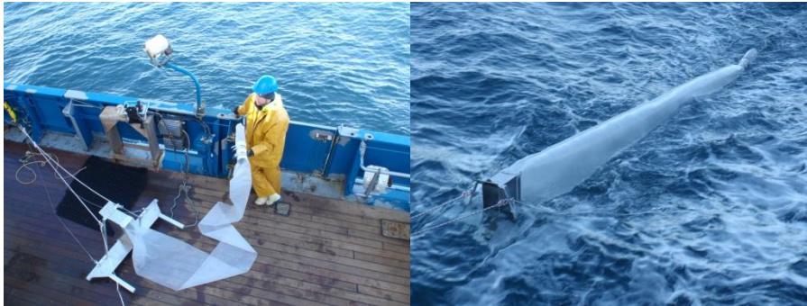
Fig. 3. A high-speed Manta trawl. (© Crown copyright 2011, permission granted by Cefas)
