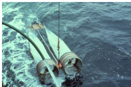
Fig. 4. A double paired horizontal bongo net.
