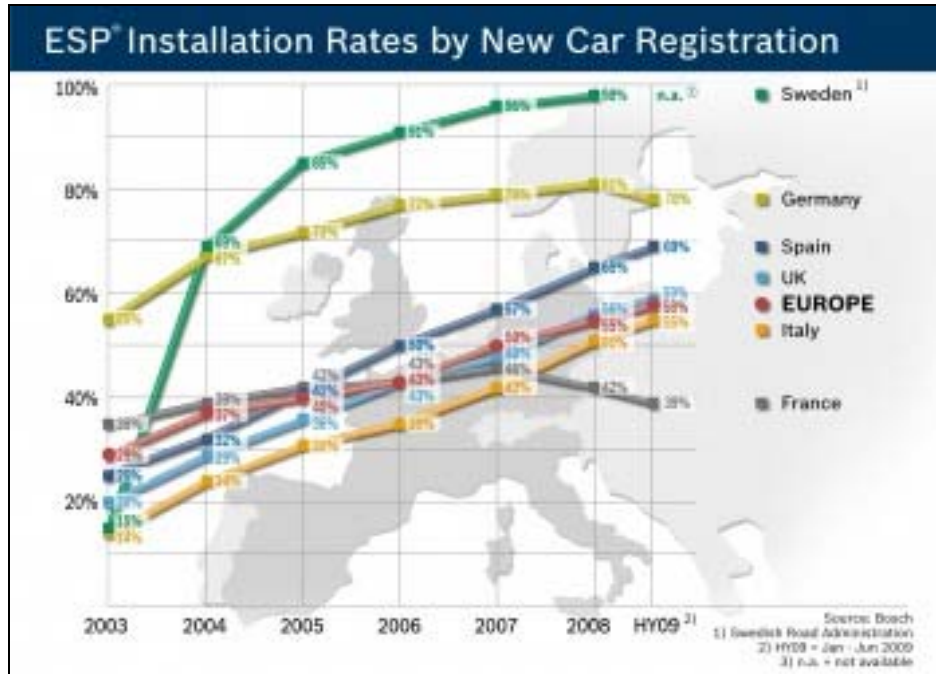
Fig. 26 INSTALLATION RATE OF ESC, JAN–JUNE 2009
