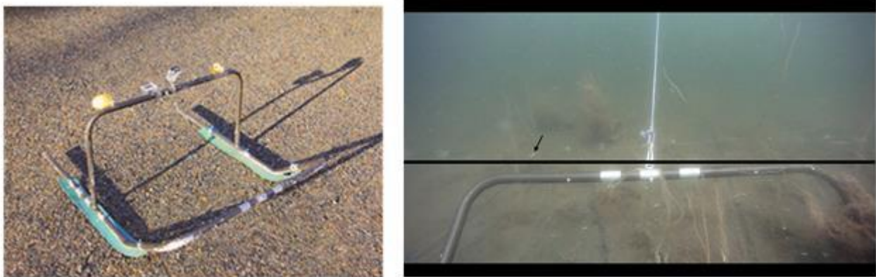
Picture 1: (Right) - The rig with two video cameras for monitoring seafloor litter. The rig was towed after a small open boat (after Lundqvist, 2013); (Left) - The method used by Lundqvist for estimating the width of a video transect. The arrow shows one of the markings (2 cm across) on the line used to calculate the width. The distance between two markings is 0.2 m and at the black line across the picture the estimated transect width is 2.55 m.
