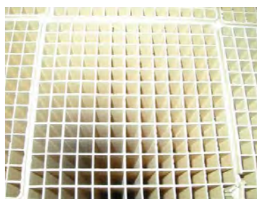
Figure 1.67: Example of an individual catalyst used for the SCR technique
