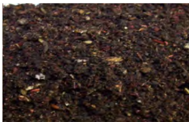
Figure 1.7: Hazardous waste – impregnated sawdust
