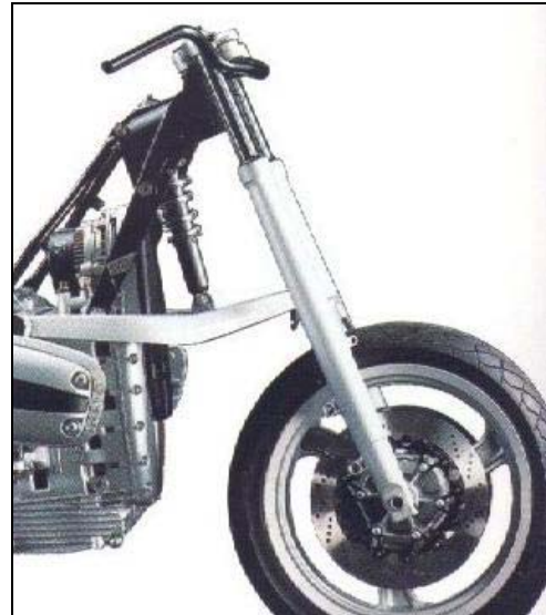
Fig 3.14: Telelever wheel control assembly [35]
