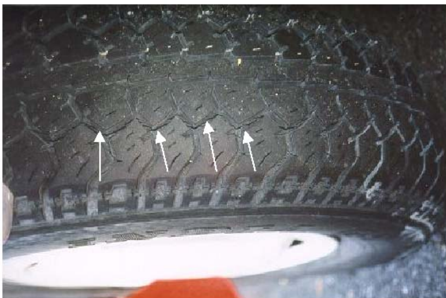
Fig. 2.6: Aging defects (e.g. cracks)
