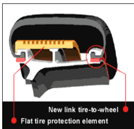
Fig. 3.4: Continental Wheel System CWS [16]
