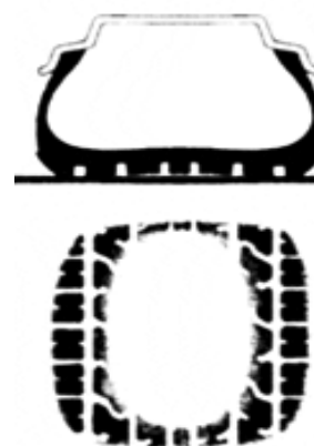
Fig. 2.14: Cross-section and footprint of an under-inflated tyre [12]
