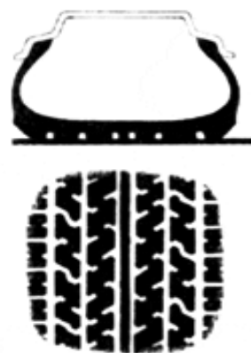
Fig. 2.12: Cross-section and footprint of a correctly inflated tyre [12]
