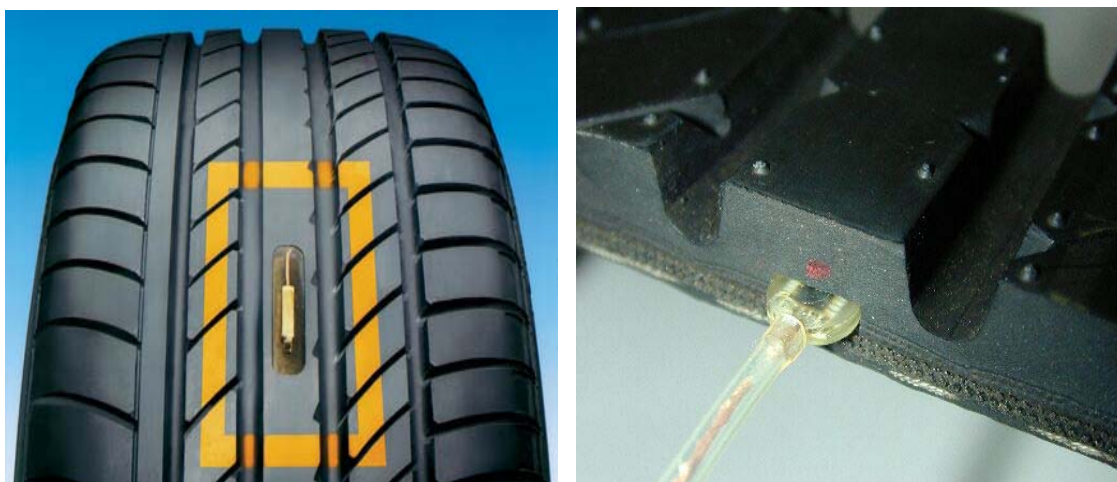
Fig. 3.9 and 3.10: SAW, vulcanised into the tyre tread [24]
