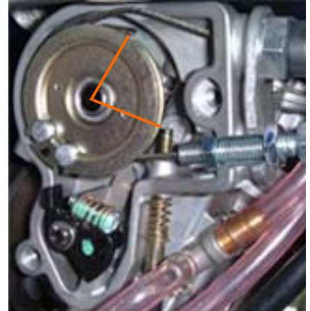
Fig. 2.12: Throttle open (without throttle stop)
