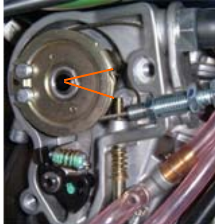
Fig. 2.11: Throttle open (with throttle stop)
