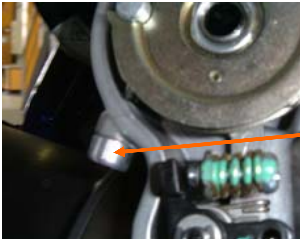
Fig.. 2.13: Throttle stop in carburettor
