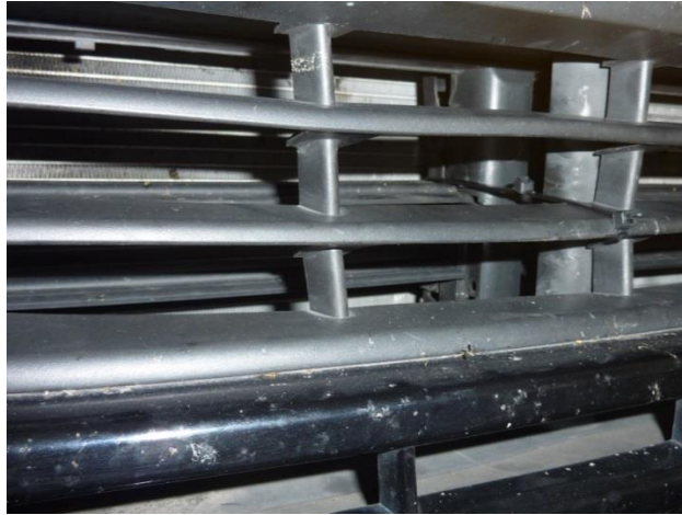
Figure 45: Active grill vanes in open position
