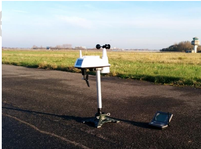
Figure 42: Davis weather monitoring system
