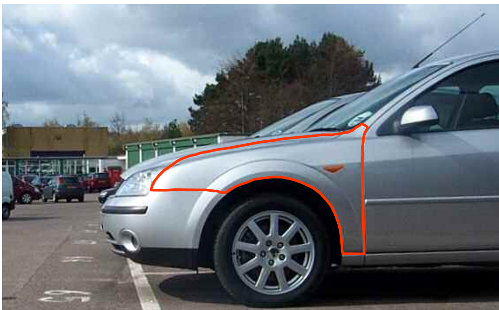
Figure 8.34. Raised wing edge to match bonnet
