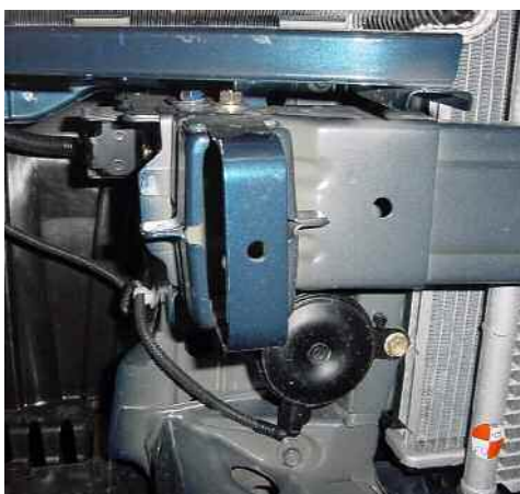
Figure 2.4. Bumper armature damage post test, L01
