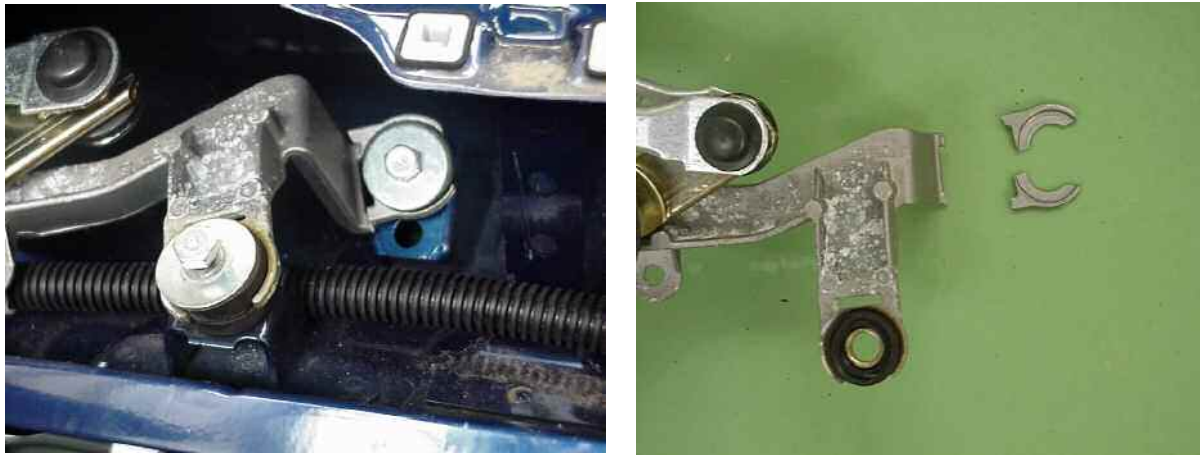
Figure 8.17. Honda Civic - frangible wiper spindle mounting following test (in place and removed)
