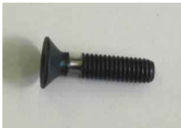
Figure 8.20. Necked shear screw - similar waisted design to be used for hinge bolt
