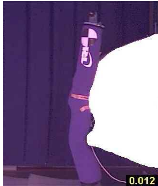
Figure 5.10. Bumper test using TRL sensor legform
