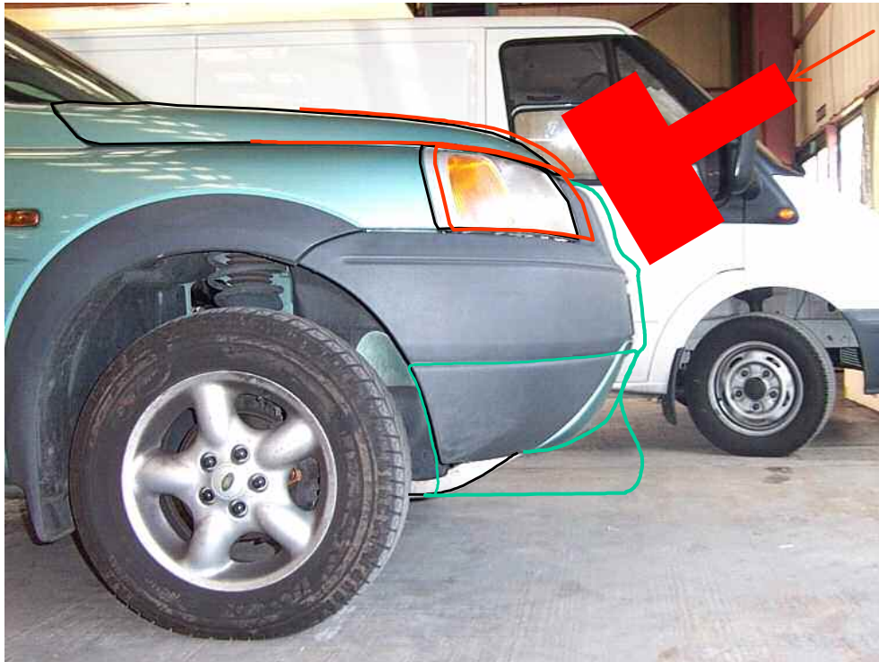
Figure 8.11. Bonnet leading edge changes following the bumper extension
