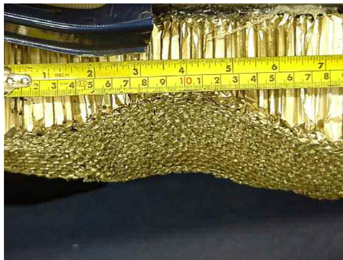
Figure 8.1. Crush of Hexcel following a pedestrian legform test
