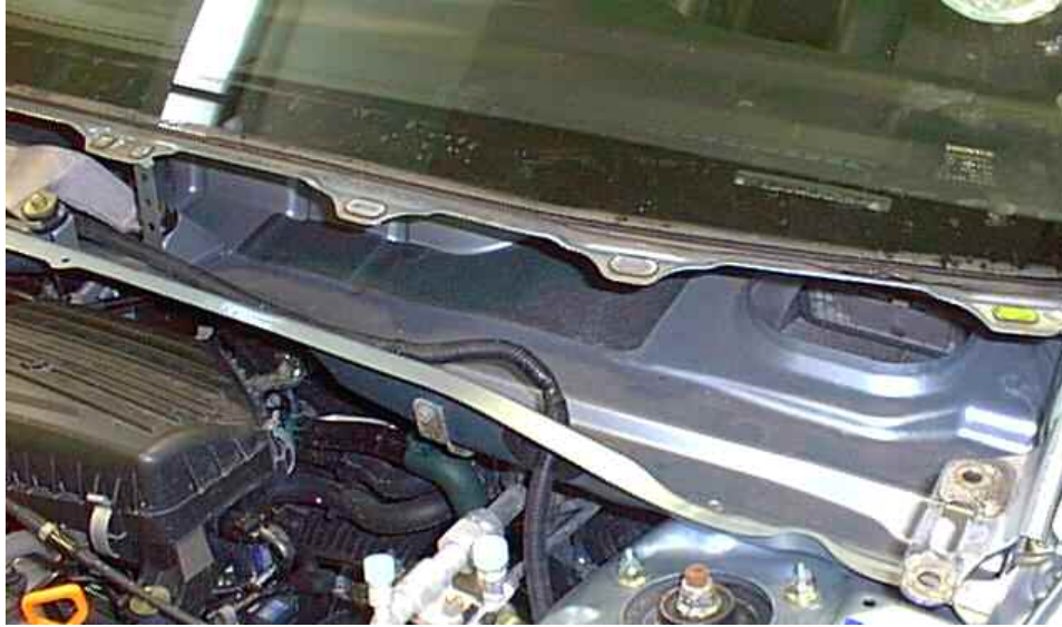
Figure 8.15. Honda Civic C-section of the upper bulkhead
