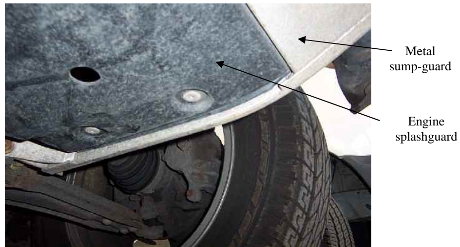
Figure 8.10. Underside of Freelander showing metal and plastic bumper support where the new spoiler would be fixed
