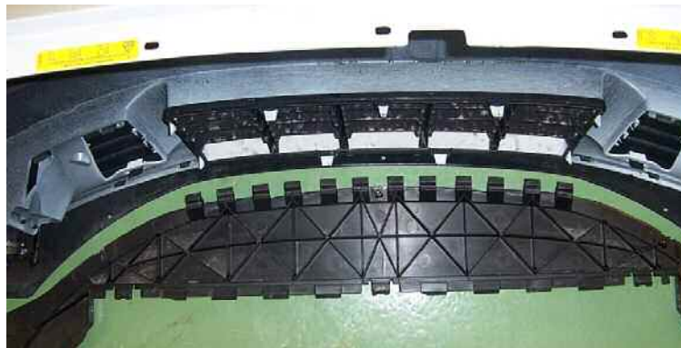
Figure 8.28. Ribbed under-tray and bumper fascia from the Volvo S40
