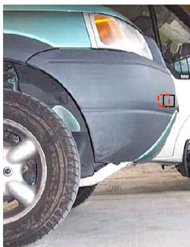
Figure 8.2. Bumper beam moved rearwards by 20 mm due to the reduction of the length of the collapsible box elements between the chassis rails and the bumper beam
