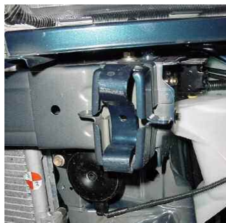
Figure 2.4. Bumper armature damage post test, L01
