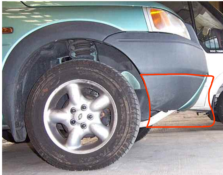
Figure 8.7. New detachable bolt-on spoiler to provide low load path for the leg
