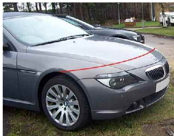
Figure 2.10. Possible adaptation or enlargement of styling change by extending plastic parts back towards red-line
