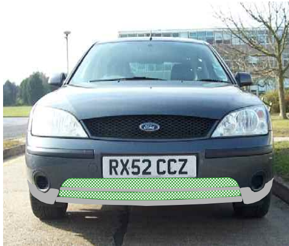
Figure 8.26. Existing bumper fascia air intake design
