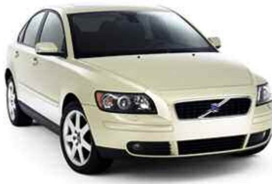
Figure 2.7. Volvo S40, with plastic front face components extending into the conventional 'bonnet' surface
