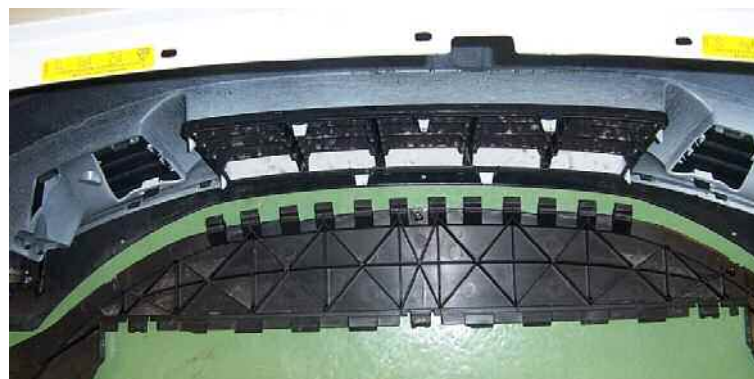
Figure 8.9. Ribbed under-tray and bumper fascia from the Volvo S40
