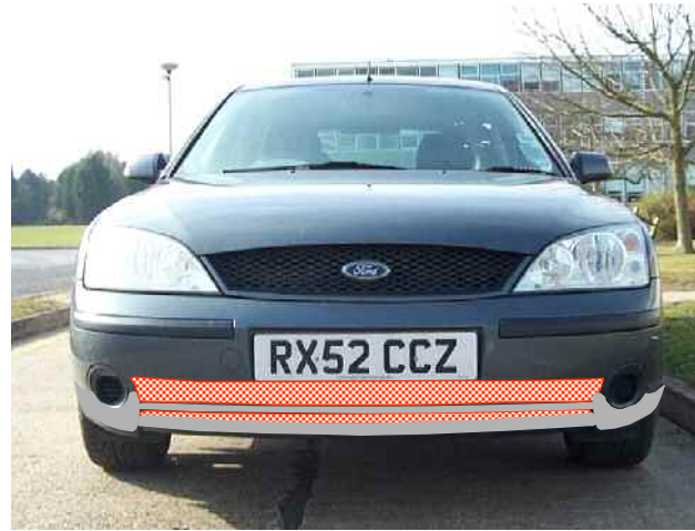
Figure 8.27. Modification to the bumper fascia required to maintain both the ramp angle and air intake area
