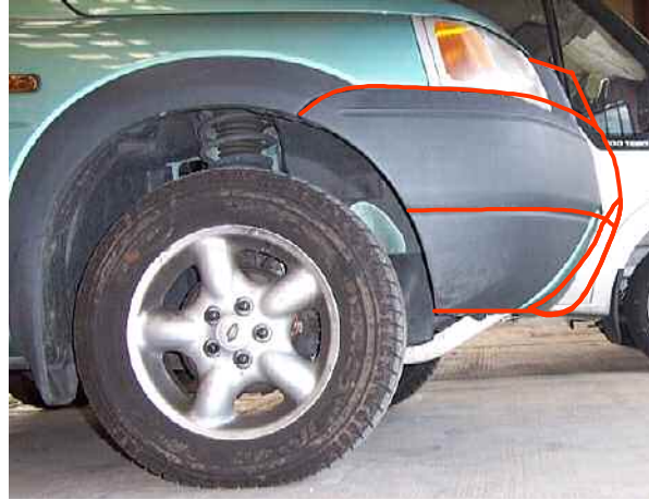
Figure 8.3. Bumper fascia moved forwards by 45 mm
