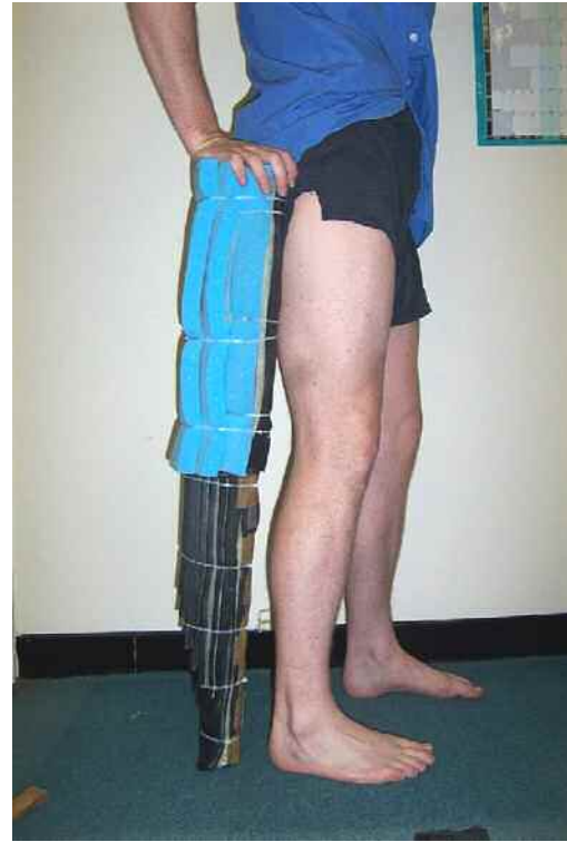
Figure 5.8. Comparison of sensor legform (skin removed) with a human leg
