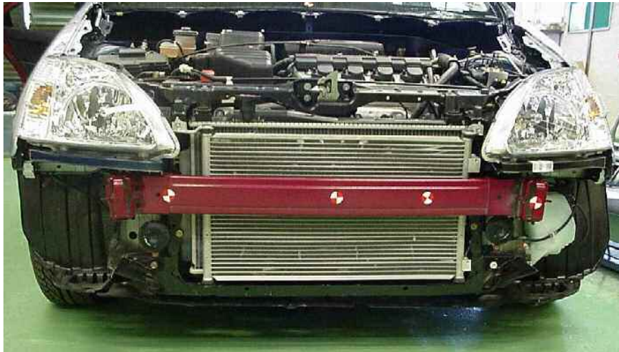
Figure 2.3. Underlying points for the legform impactor tests
