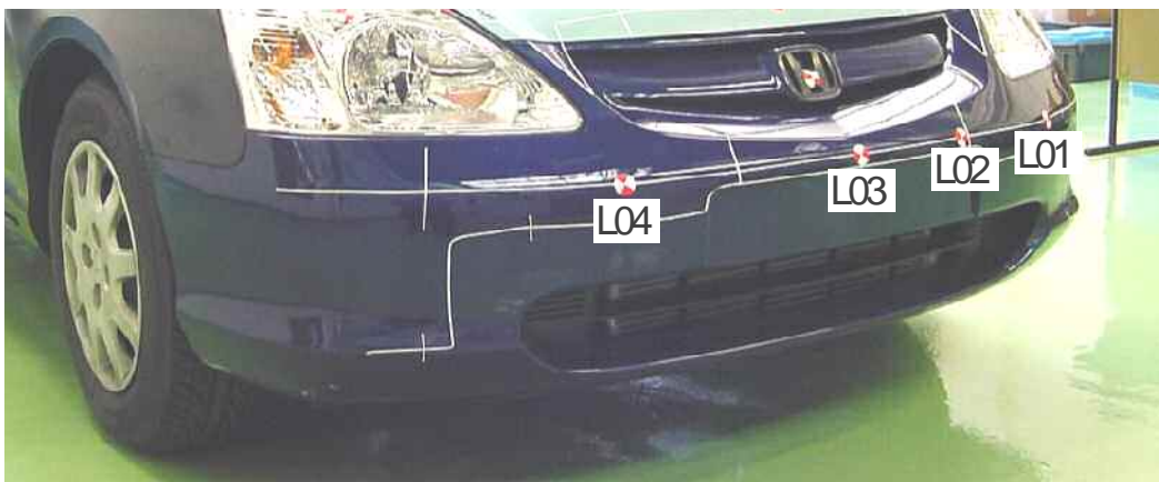
Figure 2.2. Legform test sites
