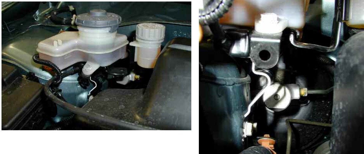
Figure 8.22. Deformable brake fluid reservoir of the Honda Civic
