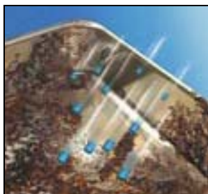
Figure 12 Granulates to foster the cleaning process
