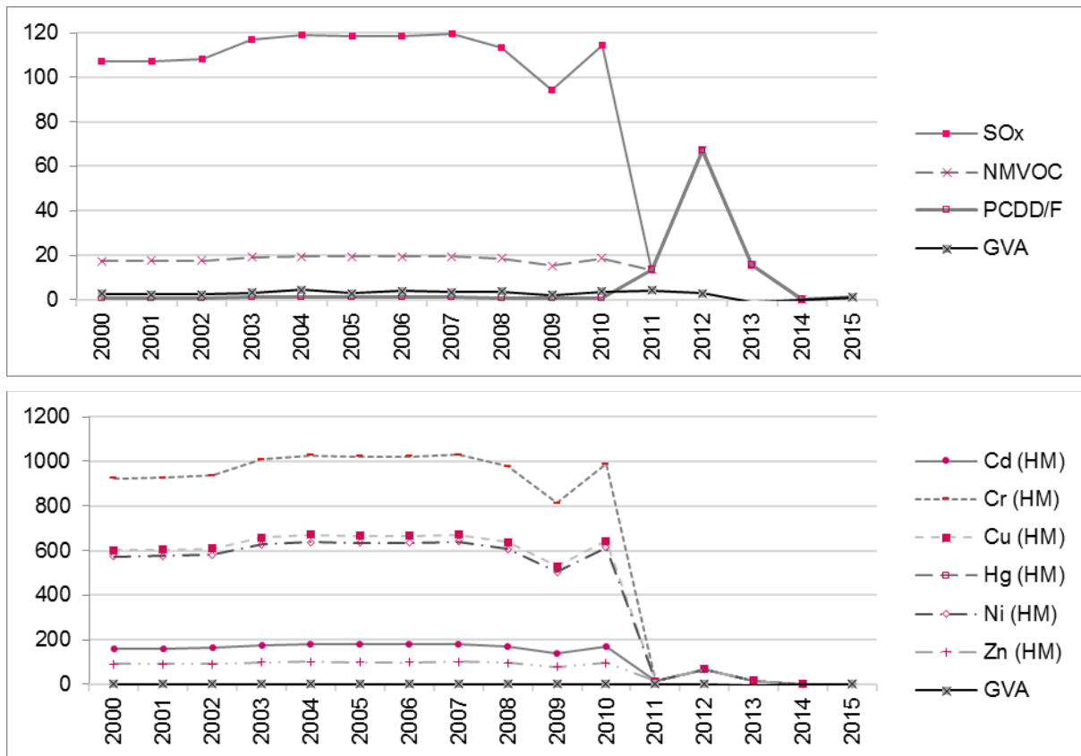
Figure 17: Indexed emissions to air from iron and steel sector (indexed to 2015=1), with outliers removed
