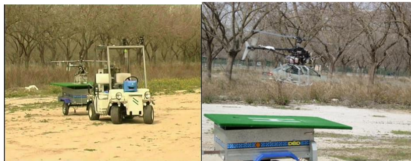
Fig. 3: CROMAT project on the coordination of aerial and ground unmanned aerial vehicles. Left the autonomous helicopter HERO being transported by the unmanned ground vehicle ROMEIO 4R. Right, landing of HERO on ROMEIO 4R.
