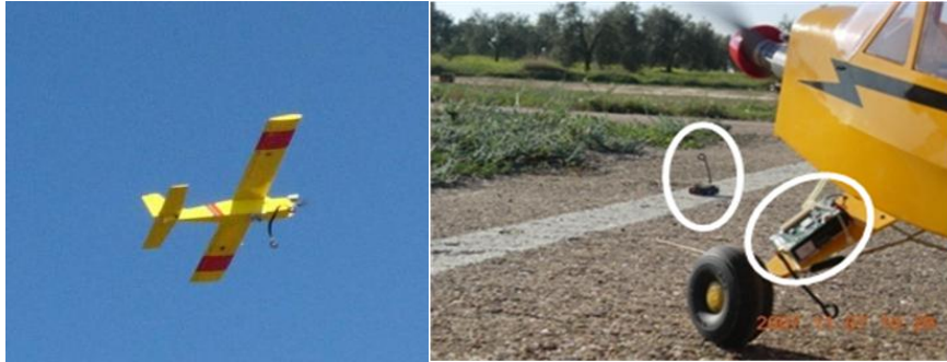
Figure 4: Fixed wing UAV developed in AEROSSENS with a node of the wireless sensor network.
