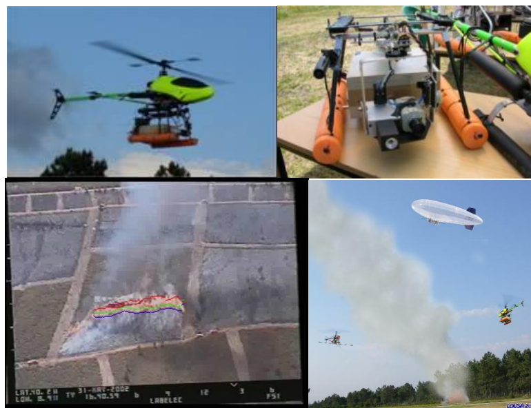
Fig.1: COMETS FP5 project: Unmanned helicopter with visual and infrared cameras monitoring and obtaining measurements of a fire.
