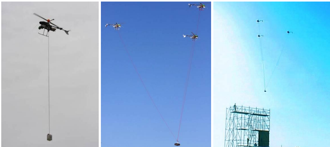
Fig. 2: AWARE load transportation with one (left) and multiple (centre) unmanned helicopters. Deployment of the load on the top of a structure simulating a building.
