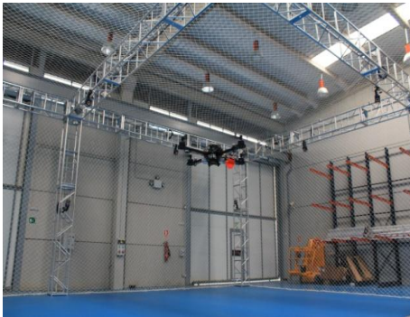
Indoor testbed with the VICON system
