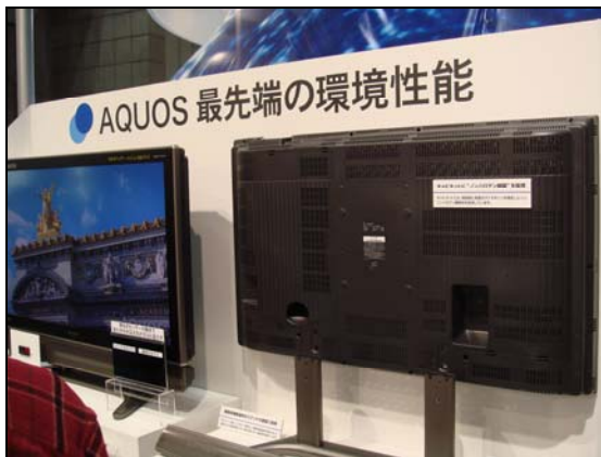
Halogen-free PE housing and bio-painted stand (Eco-Products 2006, Tokyo, Japan)
