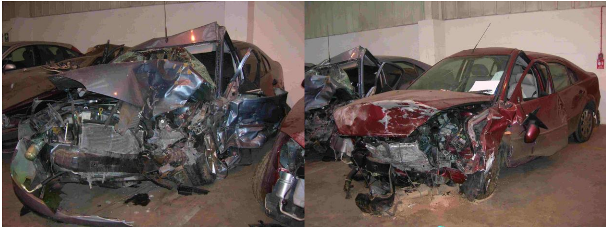
Figure 6-1. Example of car-car impact where the longitudinal did not crush as in the test
