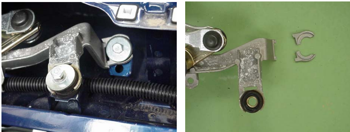
Figure 11.17. Honda Civic - frangible wiper spindle mounting following test (in place and removed)
