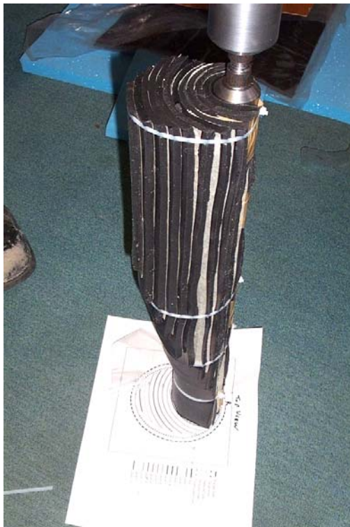
Figure 7.7. Construction of the lower leg (skin removed)
