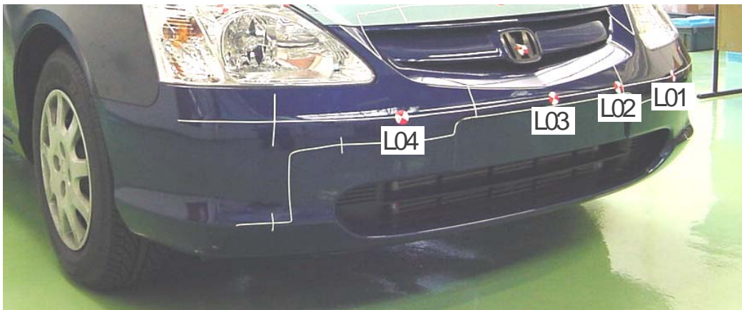
Figure 2.2. Legform test sites
