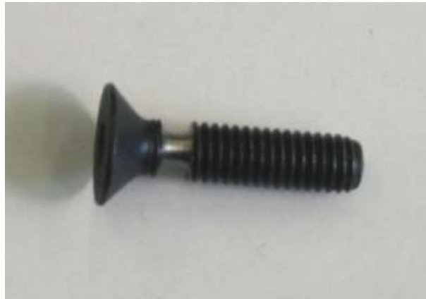
Figure 11.20. Necked shear screw - similar waisted design to be used for hinge bolt
