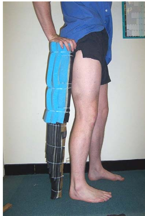
Figure 7.8. Comparison of sensor legform (skin removed) with a human leg
