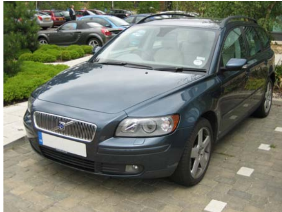
Figure 2.7. Volvo S50, with plastic front face components extending into the conventional 'bonnet' surface
