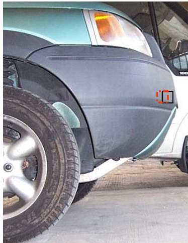
Figure 11.2. Bumper beam moved rearwards by 20 mm due to the reduction of the length of the crushable box elements between the chassis rails and the bumper beam
