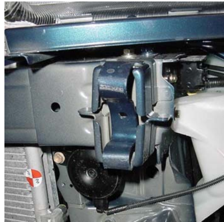
Figure 2.4. Bumper armature damage post test, L01
