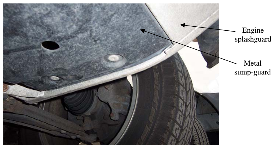
Figure 11.10. Underside of Freelander showing metal and plastic bumper support where the new spoiler would be fixed
