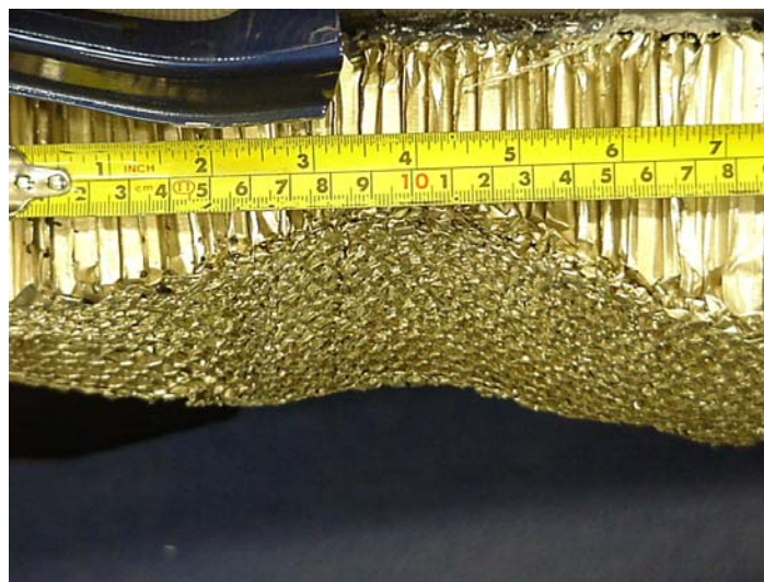
Figure 11.1. Crush of Hexcel following a pedestrian legform test
