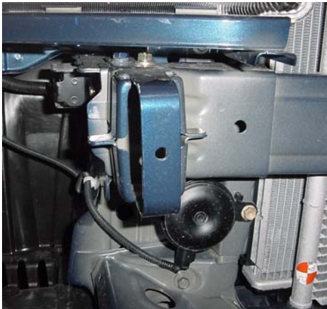
Figure 2.4. Bumper armature damage post test, L01
