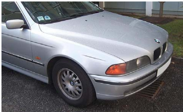
Figure 2.8. Changes in styling - older style BMW 5 Series with steel bonnet leading edge
