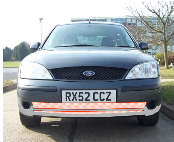
Figure 11.27. Modification to the bumper fascia required to maintain both the ramp angle and air intake area
