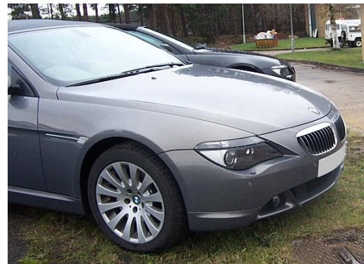
Figure 2.9. Changes in styling – new style BMW 6 Series with bumper/grill extending into bonnet, with more rounded edge
