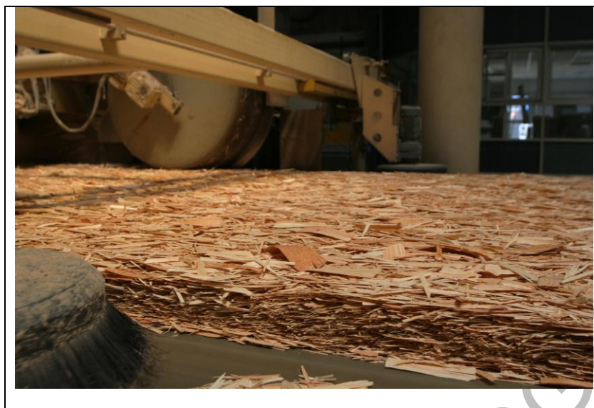
Figure 2.8: OSB mat after forming and trimming
