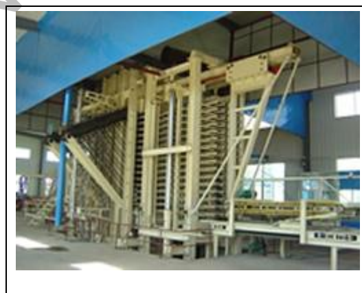
Figure 2.10: Multi-opening press and semi-enclosing suction hood
