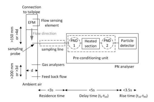
The PN analyser shall be connected to the sampling point via a sampling probe which extracts a sample from the centreline of the tailpipe tube. As specified in point 3.5 of Appendix 1, if particles are not diluted at the tailpipe, the sampling line shall be heated to a minimum temperature of 373 K (100 °C) until the point of first dilution of the PN analyser or the particle detector of the analyser. The residence time in the sampling line shall be less than 3 s.
