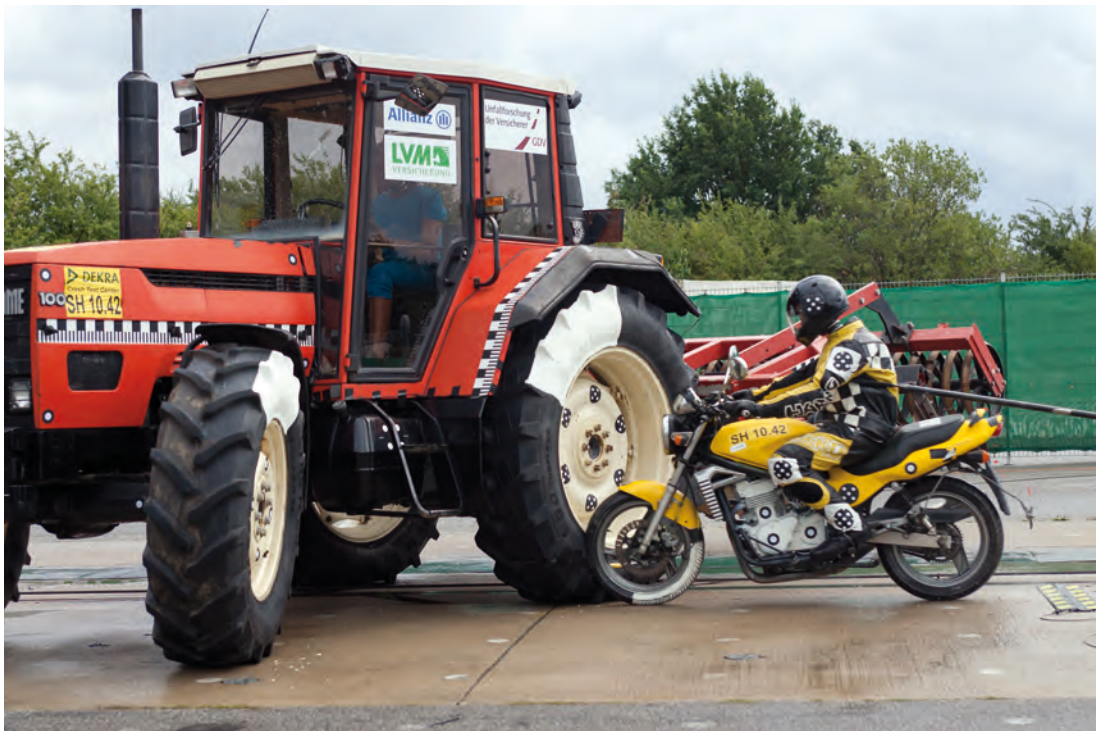
Picture 11: Crash test with tractor vs. motorbike (after the impact)
