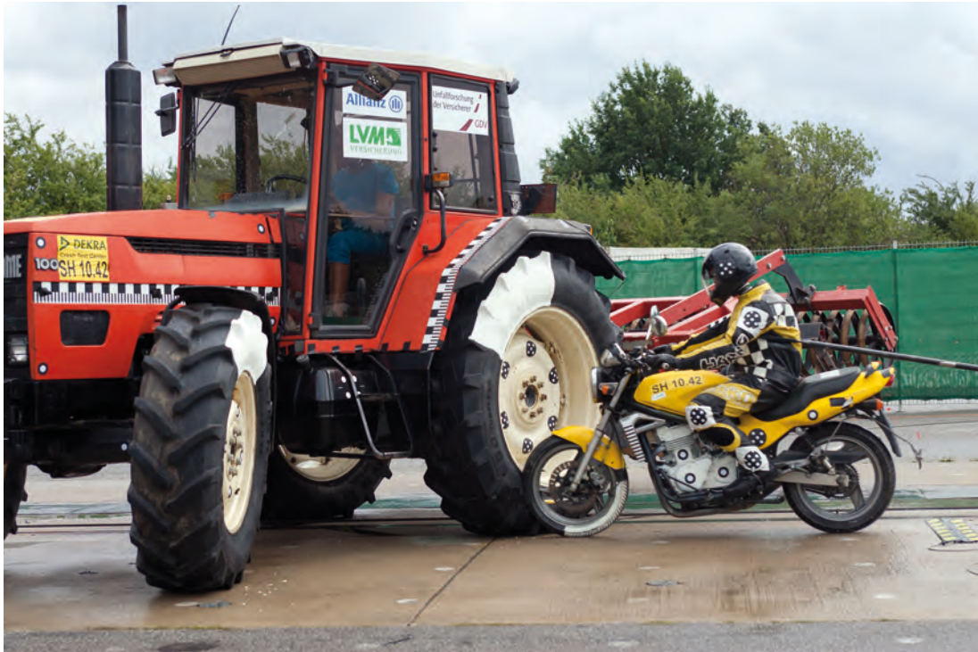
Picture 10: Crash test with tractor vs. motorbike (before the impact)
