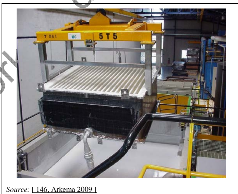
Figure 4.2: View of the deposition of an asbestos-free diaphragm on a cathode
