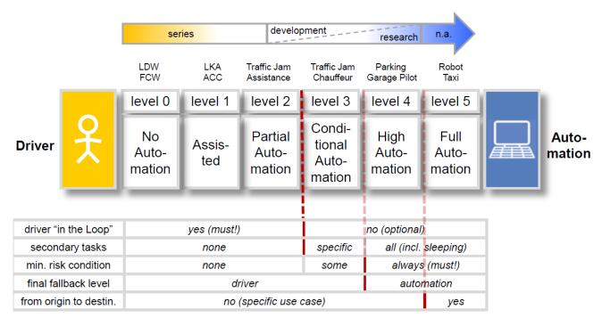
ACC: Automatic Cruise control FCW: Forward collision warning LDW: Lane departure warning LKA: Line keeping assist
