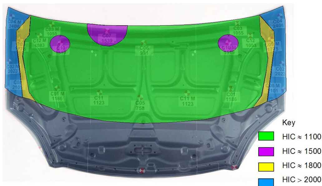
Figure 6.6. Results of testing the 2001 Honda Civic at 40 km/h with a 2.5 kg child headform (Lawrence et al. , 2002)
