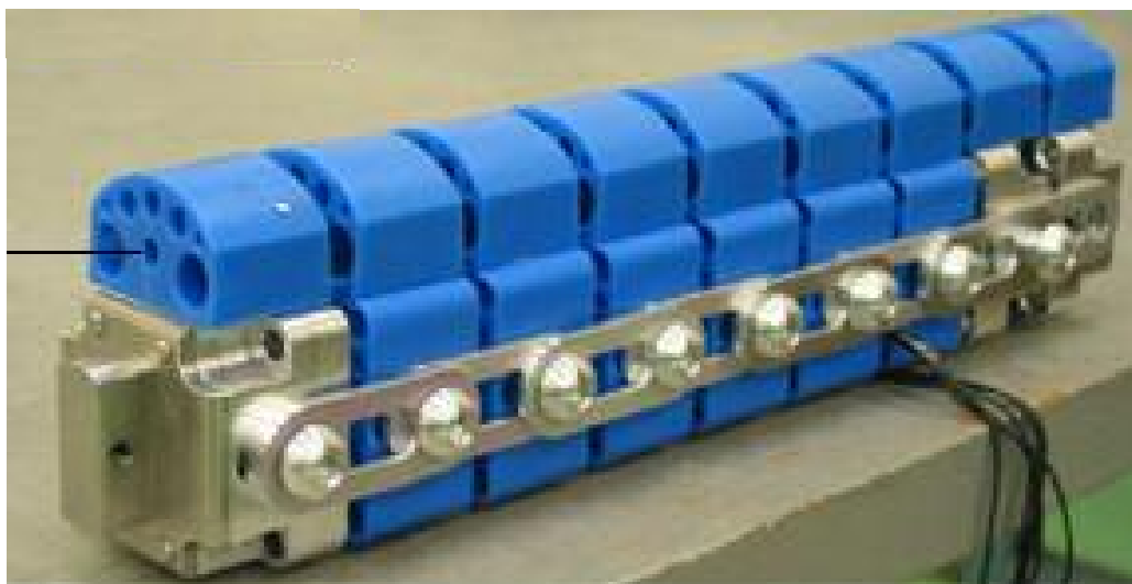
Figure 3.2. Photograph of one long bone of Flex-PLI GT \alpha showing segmental design and nylon impact face (Konosu, 2006a)
