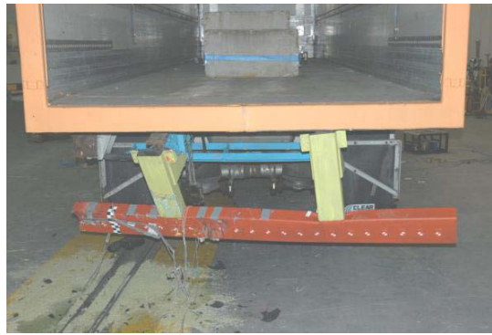
Figure 3-7. Rear view of RUP
