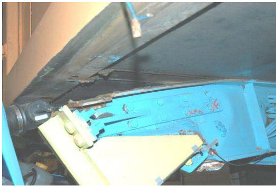
Figure 3-6. Deformation of left hand chassis beam (blue)
