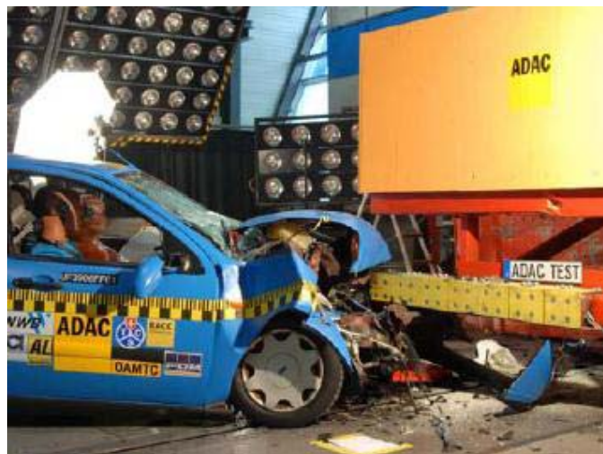
Figure 3-10. Result of 2 nd ADAC test with strengthened and lowered RUP
