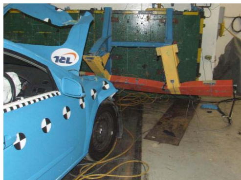
Figure 3-16. Rear view of RUP.
