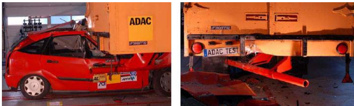
Figure 1-1. Results of ADAC crash test with underrun protection conforming to 2006/20/EC
