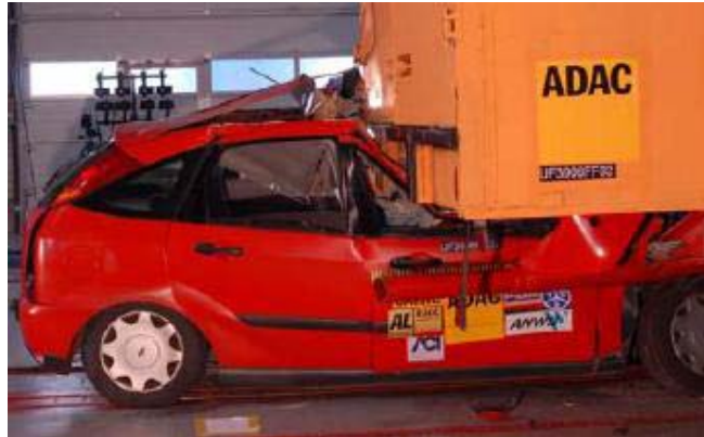
Figure 3-8. Result of ADAC crash test with RUP compliant to 2006/20/EC
