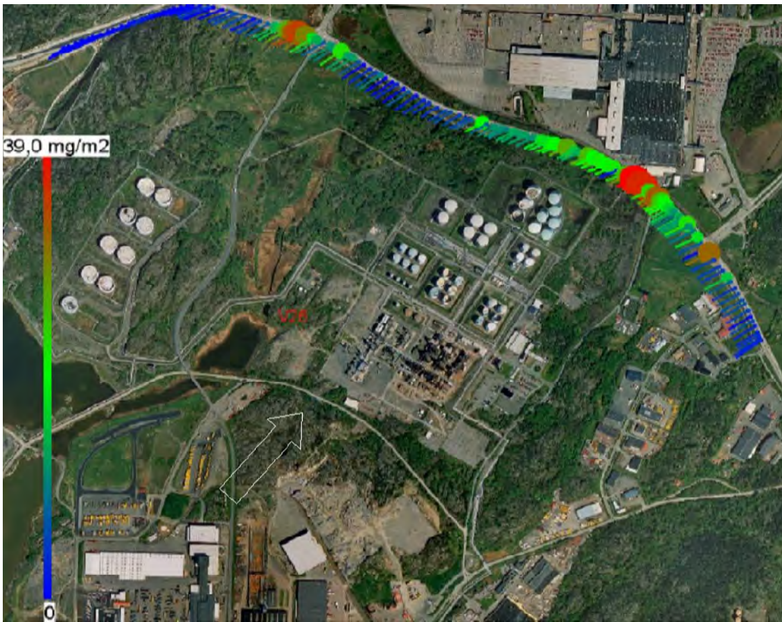
Figure 3.43: Overall shape of alkane emissions from an oil refinery as measured with SOF (the white arrow indicates the wind direction)
