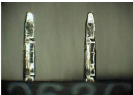
Figure 23 Types of compliant pin connector systems (Gensch et al. 2009)
